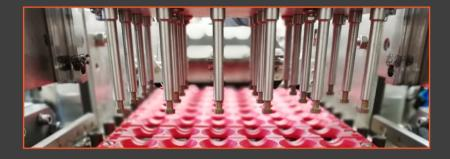
Exclusive setting system to adjust on a easyest way the chucks in order to perform the "After Pitting" prune appearance
